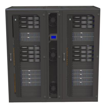
The new generation of CoolTeg air conditioning units, called **CoolTeg DXSmall**, is designed mainly for small applications. These units with a controllable cooling capacity between 3 and 7 kW can be connected to one or more IT racks. This allows them to maintain the correct conditions inside IT cabinets with heat loads ranging from 1.5 kW to 7 kW per cabinet. The typical setup includes an opened or closed system cooling unit with one or two side-positioned IT racks.
